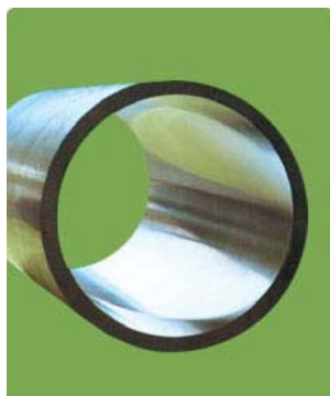
Inside honed or skived & roller burnished pipes in cold-drawn seamless ST 52 BK+S steel tol.H8 EN 10305-1 E355+SR
