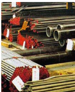
Pipes for oleodynamic circuits in cold-drawn ST 37.4 NBK steel EN 10305-4 E235+N
